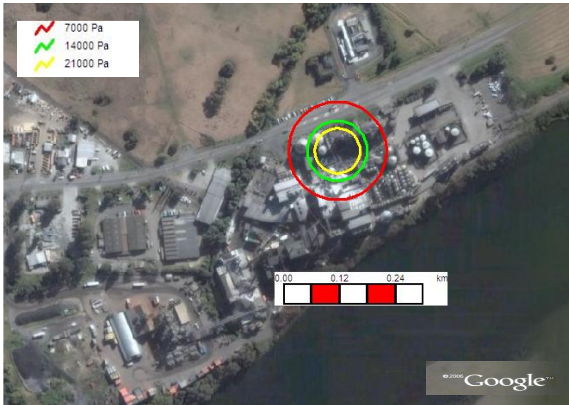
Figure C 2 Ethanol Vapour Explosion Overpressure for the Molecular Sieve
